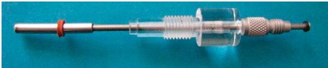
Fig. 6 –The mounting tube with the gasket slides over the membrane sleeve.
