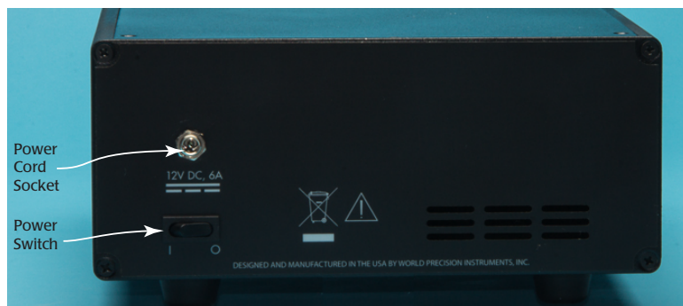
Fig. 6—The back panel has a power cord connection and a power switch.
